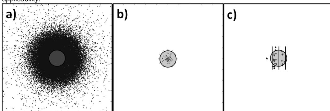
Figure 2: The use of Monte Carlo model to evaluate the protection provided by the ELPS. The location of attracted lightning on a map in three cases: a) the storage is tank unprotected; b) the storage tank is protected by lightning mast network; c) the storage tank is protected by overhead shield wires
