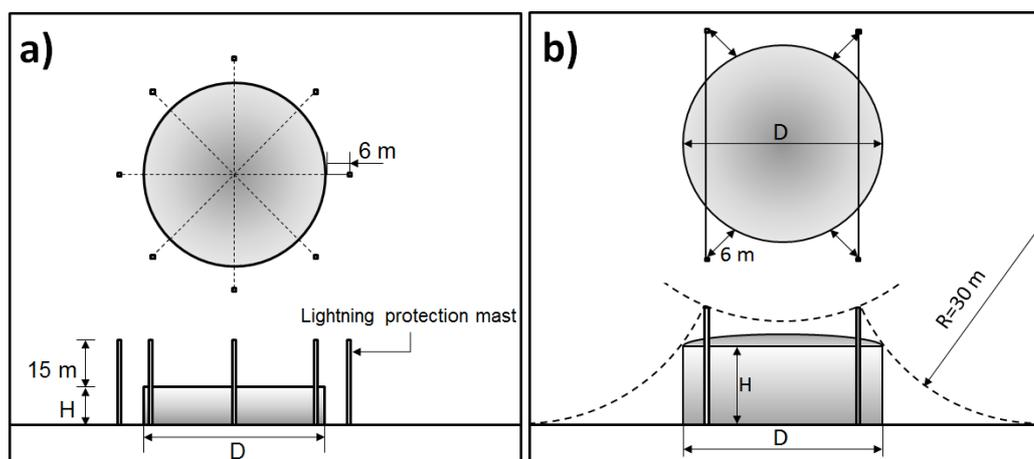
Figure 1: Air terminals for the ELPS: a) Lightning masts; b) overhead shield wire
