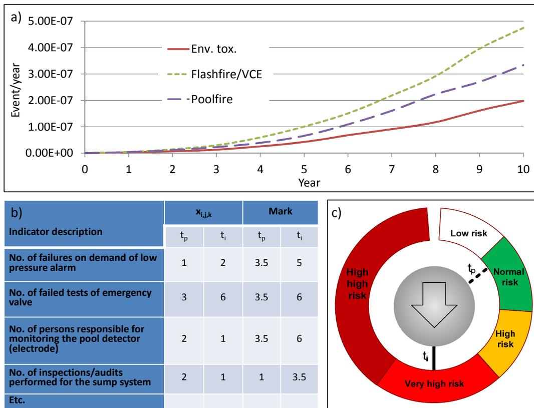
Figure 3: Preliminary results from the application of the three methodologies. a) Expected frequency of environmental damage / toxic effects, Flashfire / VCE and Poolfire calculated by means of DRA for a period of 10 years; b) examples of indicators collected at the time  $t_p$  (previous time period) and  $t_i$  (instantaneous); c) risk barometer showing the risk level at the time  $t_p$  and  $t_i$ .
