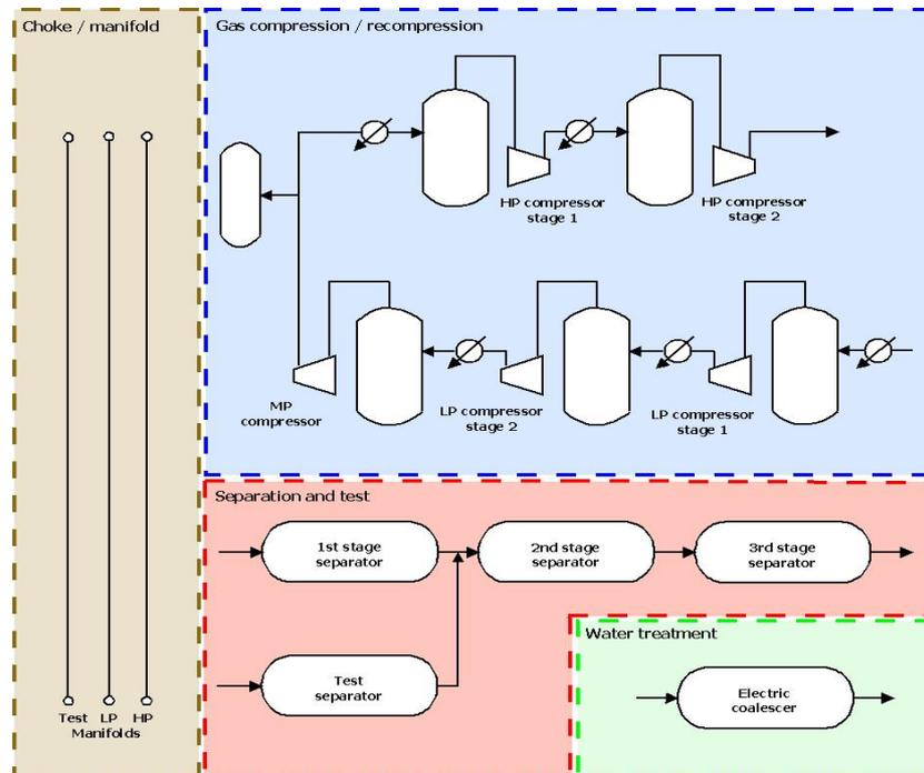
Figure 2: Generic offshore oil production process area
