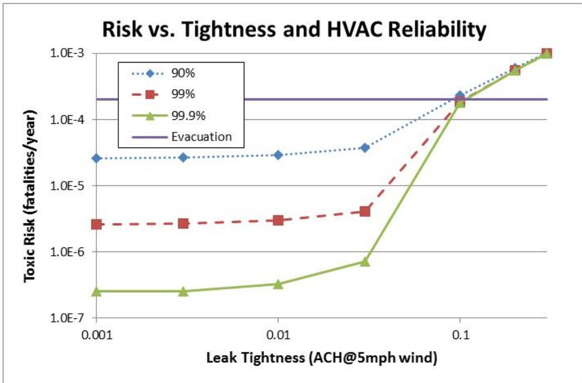
Figure 1: Toxic Risk as a Function of Leak Tightness and HVAC Isolation Reliability
