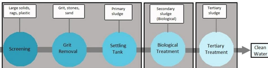
Figure 1: Flow-chart wastewater treatment process
