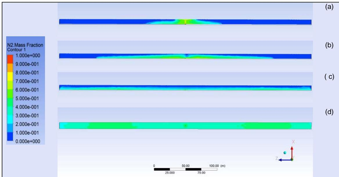
Figure 3: nitrogen concentration for case B: along the middle longitudinal plane of the tunnel: (a) after 30 s; (b) after 60 s, (c) after 120 s; (d) on the tunnel pavement: after 120 s.
