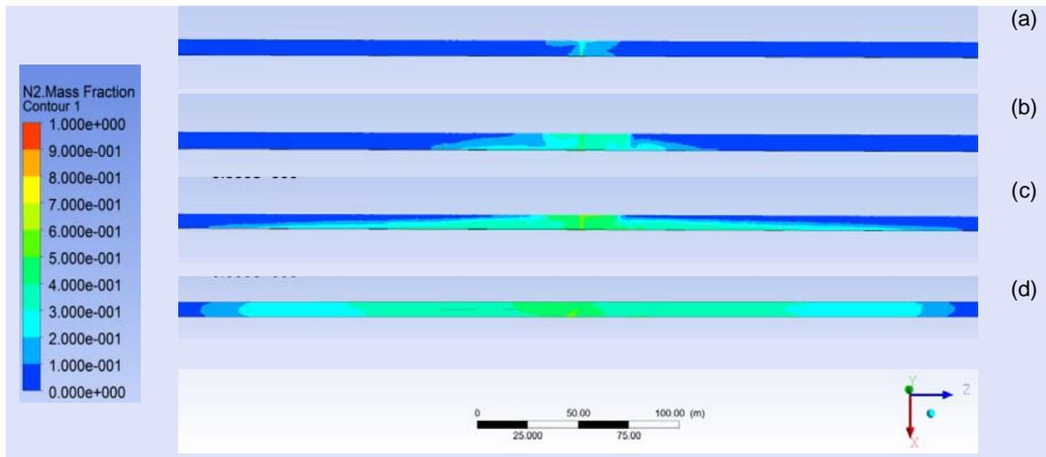
Figure 2: nitrogen concentration for case A: along the middle longitudinal plane of the tunnel: (a) after 8 s; (b) after 60 s, (c) after 120 s; (d) on the tunnel pavement: after 120 s.
