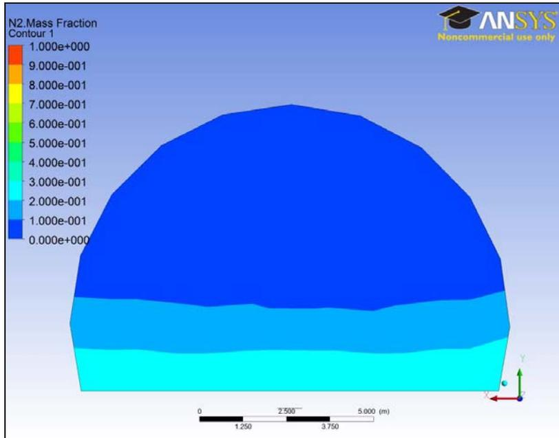
Figure 4: nitrogen concentration for case B after 120 s at the tunnel portals.
