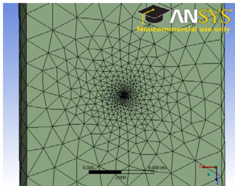
Figure 1: mesh in the proximity of the 0.25 m hole (case A).
