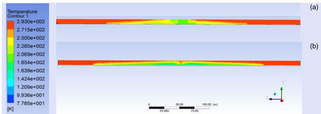
Figure 5: temperature profiles for along the middle longitudinal plane of the tunnel after 60 s; (a) case A; (b) case B.
