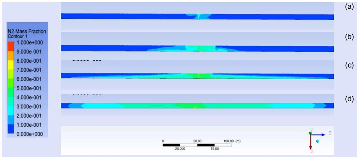
Figure 2: nitrogen concentration for case A: along the middle longitudinal plane of the tunnel: (a) after 8 s; (b) after 60 s, (c) after 120 s; (d) on the tunnel pavement: after 120 s.
