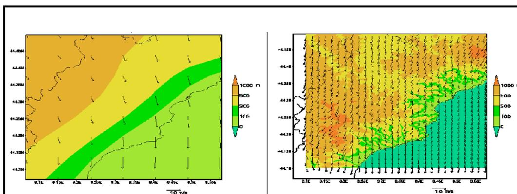
Figure 2: Wind field modelling by SafeAirII
