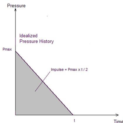
Figure 1: Idealized Blast Pressure Function
