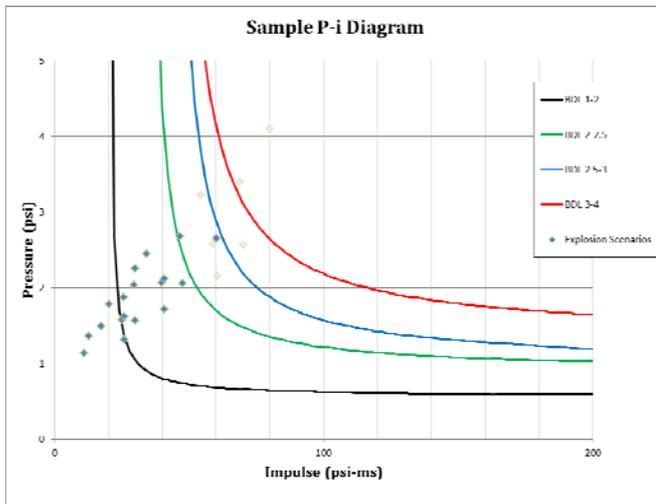
Figure 3. Example of P-i Diagram
