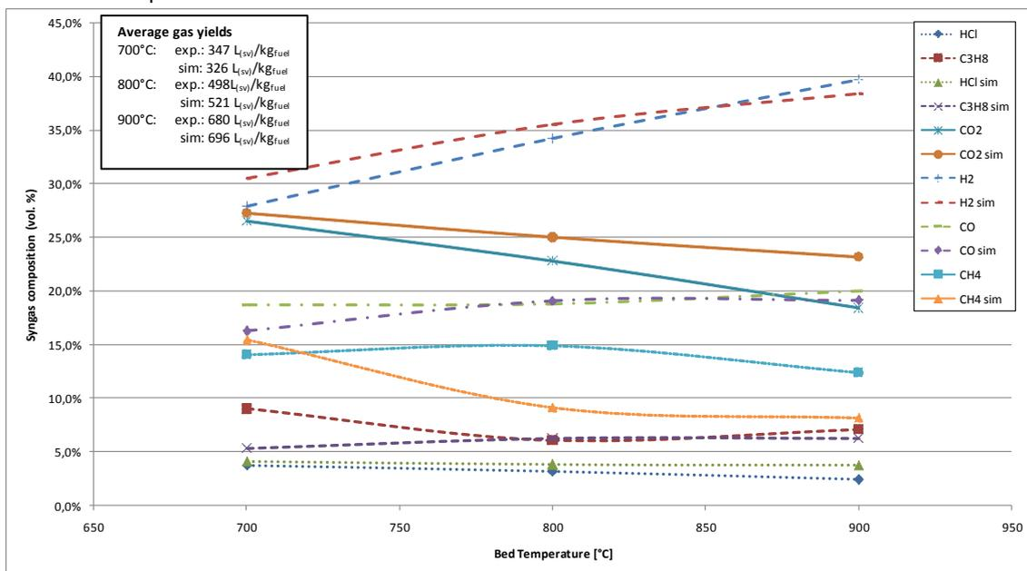
Figure 2: Syngas compositions (vol.-%) at gasification temperatures of 700 °C, 800 °C and 900 °C, experimental and simulation data
