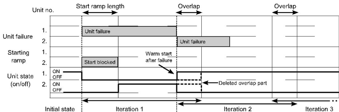
Figure 2: Forced outage simulation example
