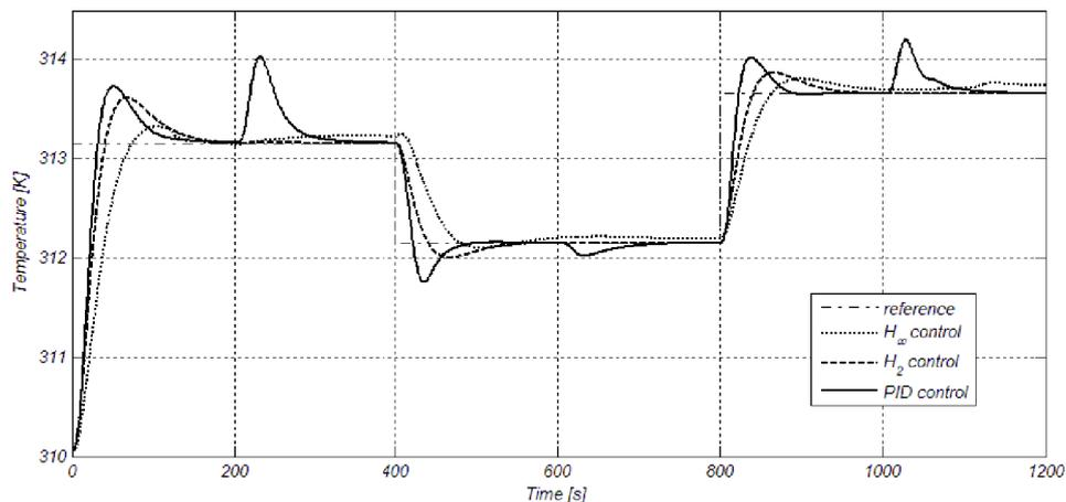
Figure 5: Comparison of the outlet kerosene temperature control
