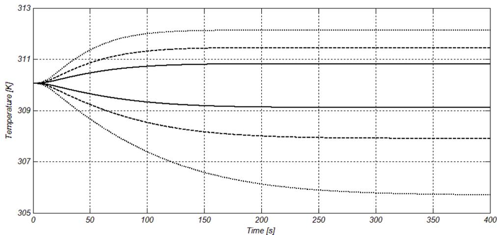
Figure 1: Step responses of the outlet temperature on the step changes of the control input
