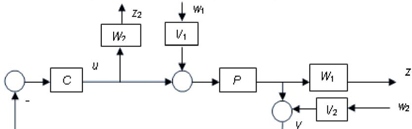
Figure 3: Generalized configuration
