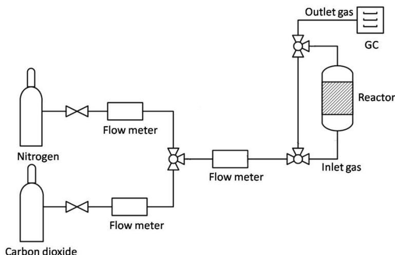
Figure 1: CO<sub>2</sub> Experiment set-up for dynamic CO<sub>2</sub> adsorption measurement
