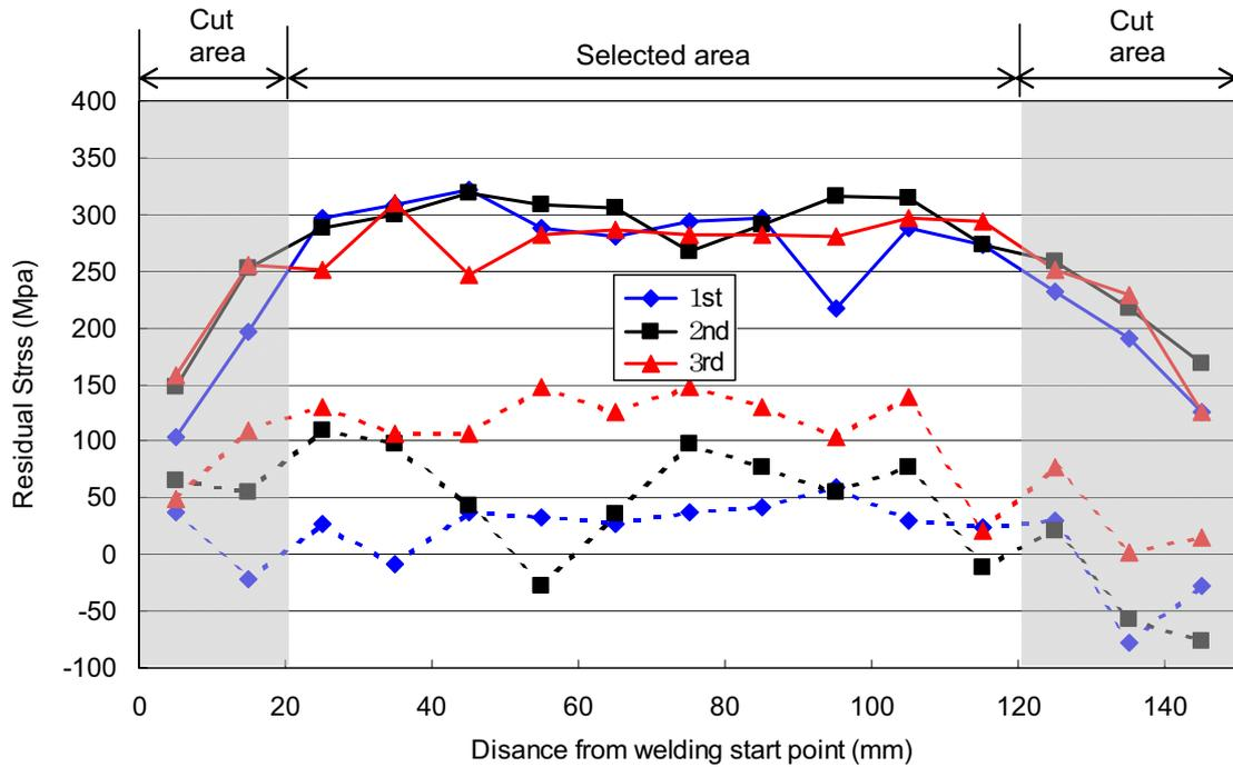
Figure 6: Residual stress using ultrasonic vibration ( $10m/s^2$ )
