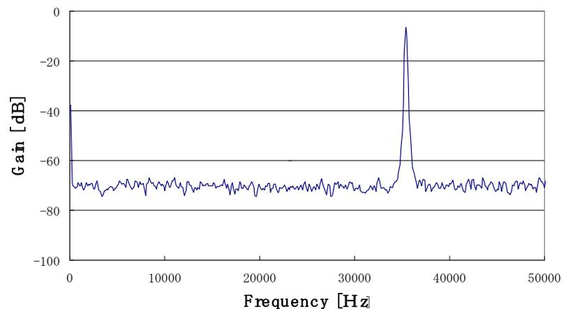
Figure 5: Power spectral density function for ultrasonic vibration
