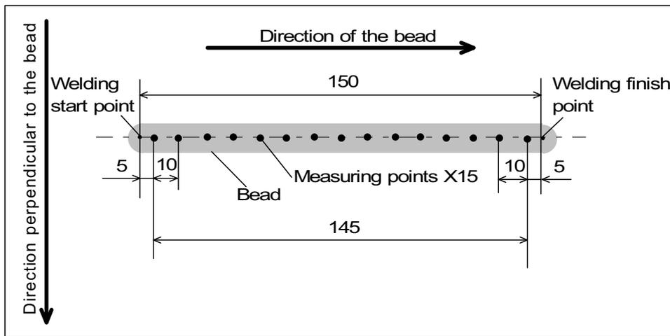
Figure 4: Measuring points of residual stress (mm)
