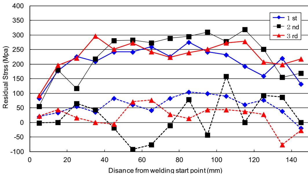
Figure 7: Residual stress using low frequency vibration (100Hz)
