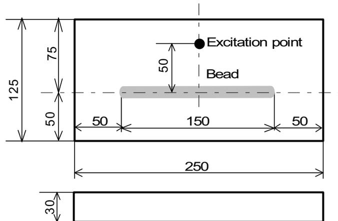
Figure 1: Size of specimen for ultrasonic vibration (mm)
