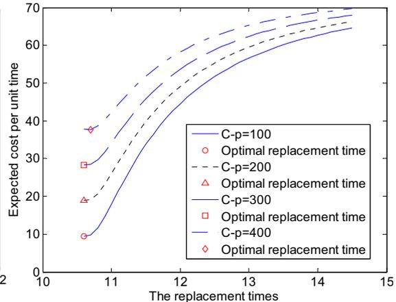
Figure 2: The expected replacement cost per unit time by Elwany's approach at  $t_k = 10.5$
