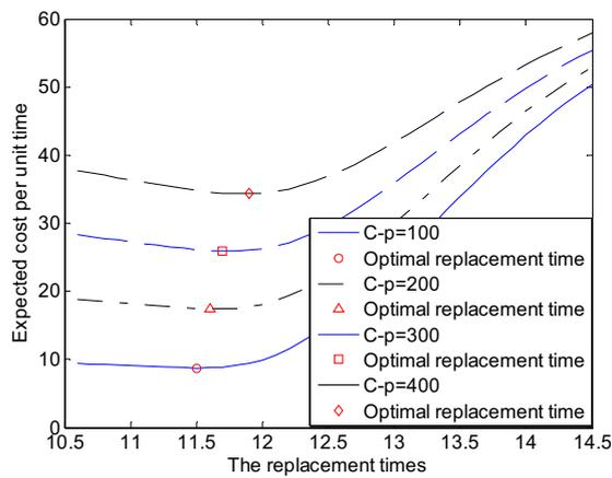
Figure 3: The expected replacement cost per unit time by our approach at  $t_k = 10.5$
