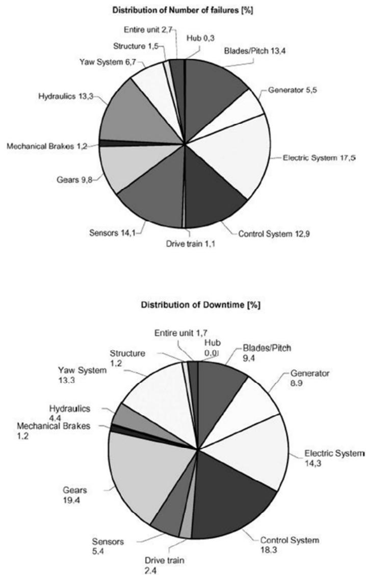
Figure 1 Comparison between downtime and number of failures (Ribrant, 2007)
