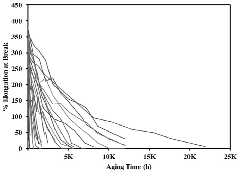
Figure 2: Elongation at Break (EAB) Data of CSPE Jacketed Cables Extracted from the CPAD
