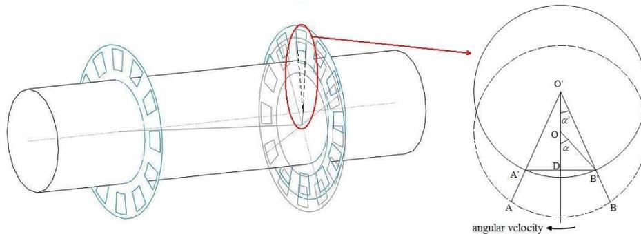
Figure 4: Diagram for decentred error of coding wheel
