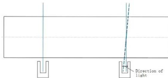
Figure 5: Diagram for the tilt of coding wheel
