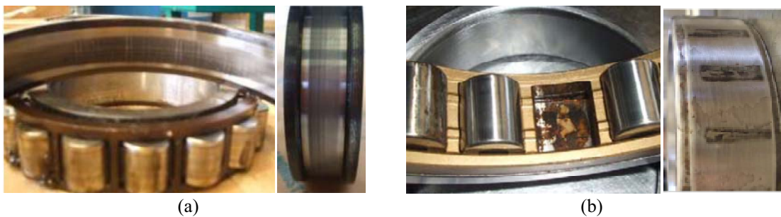
Figure 3: Cylindrical roller bearings taken from the service: (a) configuration ① - bearing at the DE side of the traction motor; (b) configuration ② - bearing at the high speed shaft of the HST gearbox.
