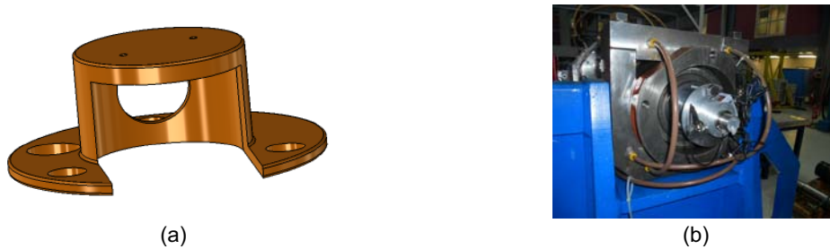
Figure 4: Custom made carter to hold the sensor and the preamplifier: a) CAD model; b) application at the axle end
