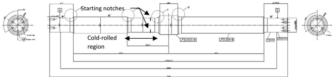
Figure 2: Drawing of the adopted full-scale specimen
