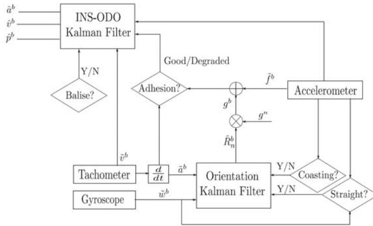
Figure 2: block diagram of the innovative localization algorithm
