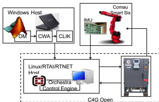
Figure 3: architecture of the HIL test rig
