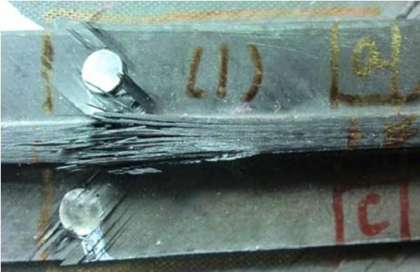
Figure 2: Partial fracture in the wing skin panel b
