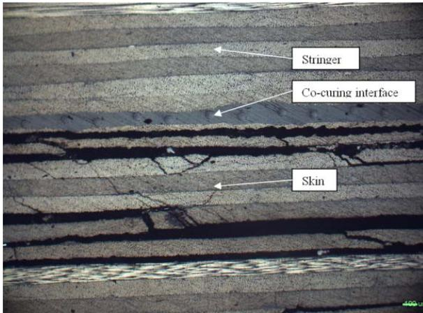
Figure 5: Region A metallographic morphology
