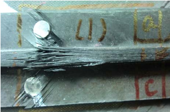
Figure 2: Partial fracture in the wing skin panel b
