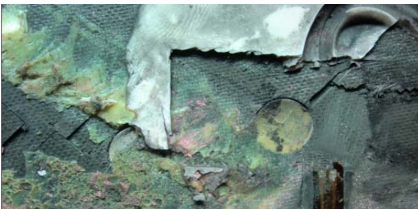
Figure 4: Stringer fracture morphology
