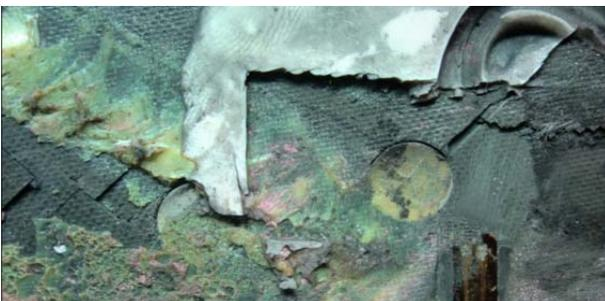
Figure 4: Stringer fracture morphology
