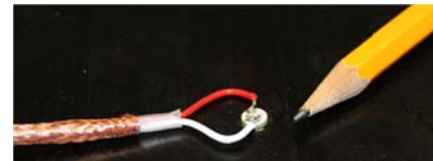
Figure 3: Detail of a surface mounted PZT transducer.
