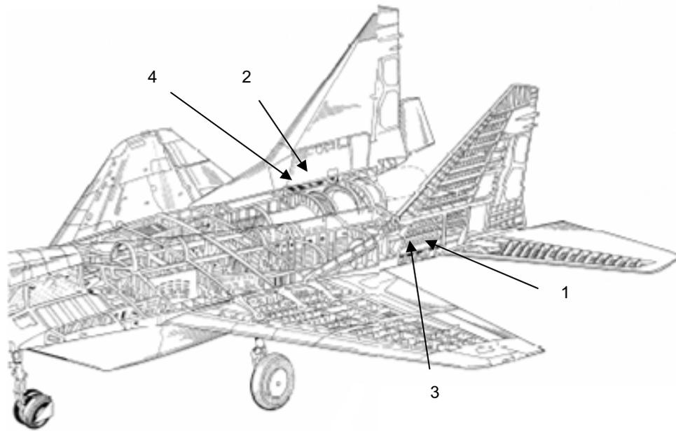
Figure 1: Strain gauges' arrangement
