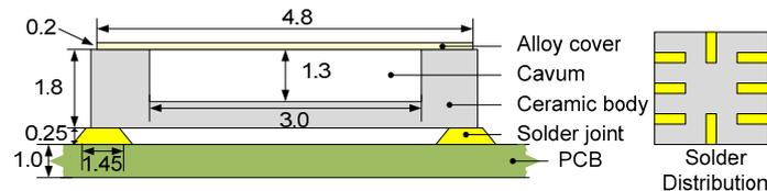
Figure 1: MEMS structure parameters
