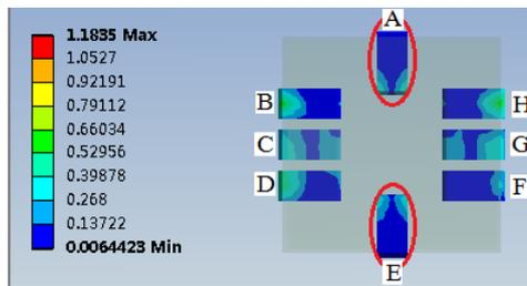
Figure 4: Random vibration analysis results (unit: MPa)
