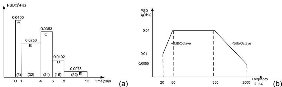
Figure 2: PSD and velocity of different pavement levels
