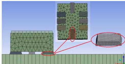
Figure 3: Finite element model of ADXL78
