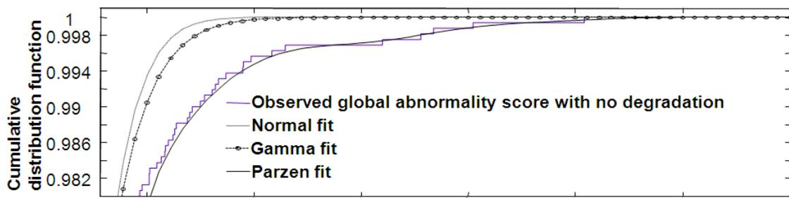
Figure 4: Observed and adjusted cumulative distribution function of ESC global abnormality score with no degradation.
