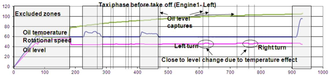
Figure 2: Engine oil consumption, EOC, oil level captures
