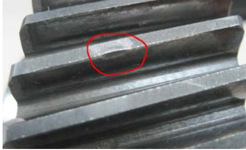
Figure 3: Gear wheel with a tiny tooth defect
