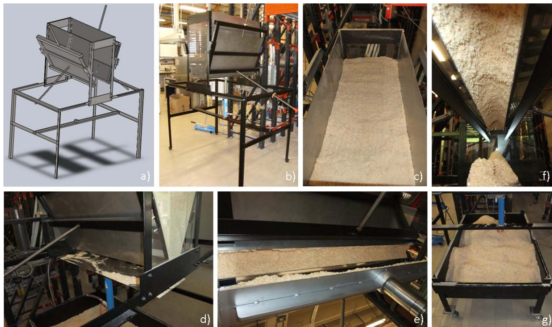
Figure 1: Experimental plane silo with variable shape a) sketch; b) full size view; c) material levelling before experiments; d) and e) silo opening; f) stable arch; g) material collected in the discharge basin.
