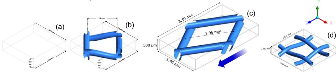
Figure 1: Unit cell for the (a) empty channel, (b) woven, (c) DelStar Naltex and (d) Deukum spacer-filled channels.
