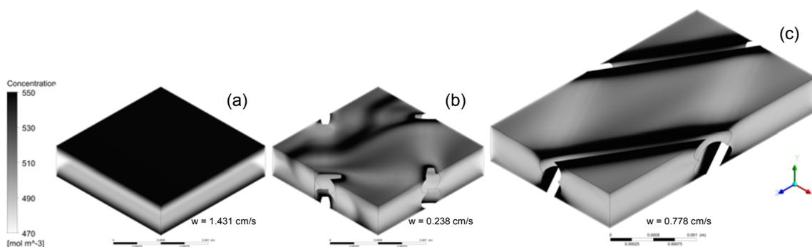
Figure 3: Concentration distribution for (a) empty channel ( $400\ \mu\text{m}$  thick), (b) woven and (c) DelStar Naltex spacer-filled channels fed by seawater at the imposed pressure drop of  $0.01\ \text{bar/m}$  and  $i = 200\ \text{A/m}^2$ .
