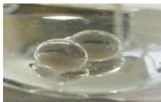
Figure 1: Two adjacent water in oil drops relying at the interface of two liquids
