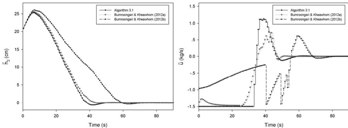
Figure 2: a) The water level in tank 2 (regulated output) and b) the water flow (control input).
