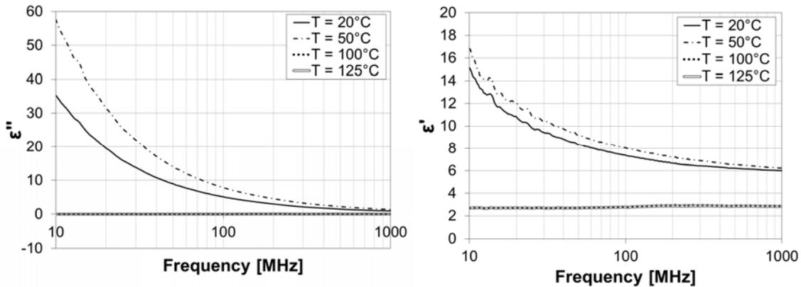
Figure 2: Measured dielectric properties of oil sand samples from room temperature up to above the connate water boiling temperature (Sarri et al., 2012).
