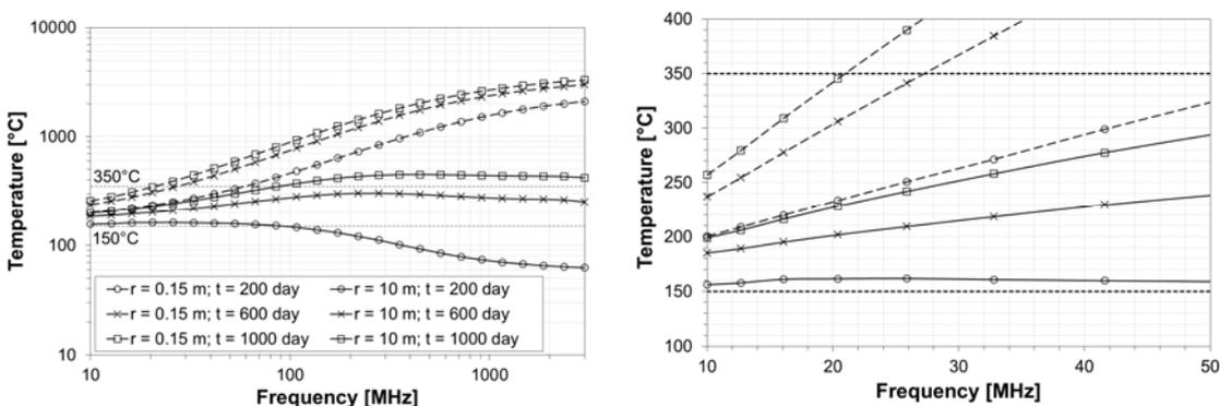
Figure 4: Frequency-temperature analysis for 200 kW irradiated power, 3 m radius tight-shell ( $\text{tg}(\delta) = 10^{-3}$ ). The diagram shows the temperatures reached at 10 m distance from the radiating well (solid lines) and near the wellbore (spotted lines) for different irradiation times, as a function of the transmitted frequency (in the range 10-3000 MHz). On the right, the range 10-50 MHz is zoomed.
