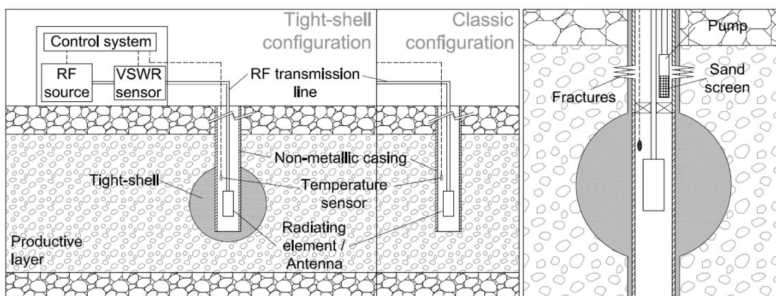
Figure 1: Scheme of the RF radiating well in the tight-shell configuration and in the classic configuration (left) and particular of a possible radiating/producing well completion with tight shell (right).
