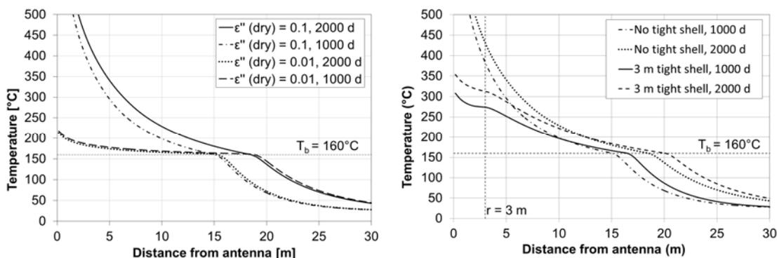
Figure 3: Simulation results. Left: comparison between thermal profiles obtained varying the dielectric properties of dried reservoir material without the use of the tight shell ( $f = 10\text{ MHz}$ , emitted power = 200 kW). Right: comparison between thermal profiles obtained without the use of the tight shell and with a 3 m radius tight shell ( $\epsilon''(\text{dry}) = 0.1$ ,  $\text{tg}(\delta)(\text{shell}) = 10^{-3}$ ,  $f = 10\text{ MHz}$ , emitted power = 200 kW).
