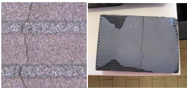
Figure 2: fractures in SiC catalysed samples.
