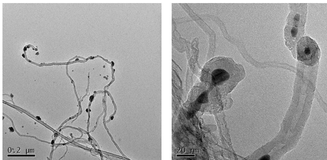
Figure 3: TEM image of pristine MWCNTs after 2700 s of reaction. Left) metallic nanoparticles are present outside the nanotubes (black particles) Right) ferrous nanoparticles (dark spots) are allocated in the tip of carbon nanotubes.
