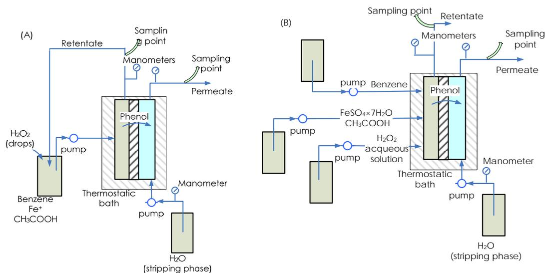
Figure 1: Scheme of semi-batch membrane (a) and continuous membrane systems (b) [Sep. Pur. Technol, 2013, <http://dx.doi.org/10.1016/j.seppur.2013.01.019>]
