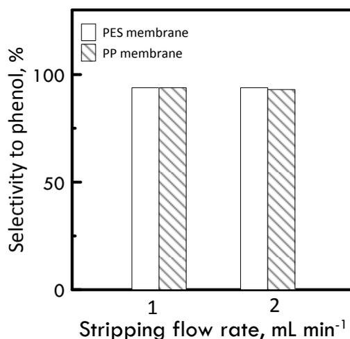
Figure 4: Selectivity permeate side using PES and PP membranes at different flow rates in the continuous membrane reactor
