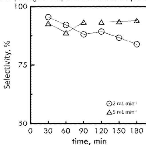
*Figure 3: Selectivity permeate side using PP membranes at different flow rates in the semi-batch system*
