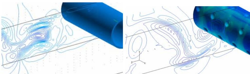
Figure 5: Comparison of the velocity distribution near the outside of a tube for a) Plain unenhanced tube and b) Vipertex 1EHT enhanced tube
