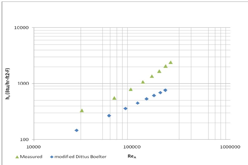
Figure 6: Comparison of the measured outside annulus heat transfer coefficient as a function of the annulus Reynolds Number for the Vipertex 1EHT enhanced tube and a smooth tube.
