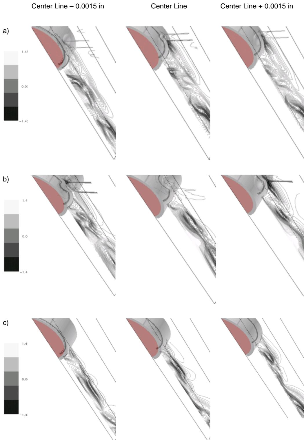
Figure 4: Comparison of the velocity distribution for (a) 0.138 in (0.351 cm) dimple enhancement, (b) 0.2 in (0.508 cm) dimple enhancement, (c) smooth tube, at various locations for the same time period.
