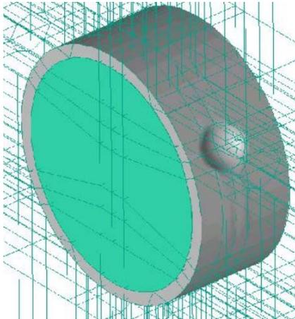
Figure 1: Sample mesh for CFD analysis of an enhancement character
