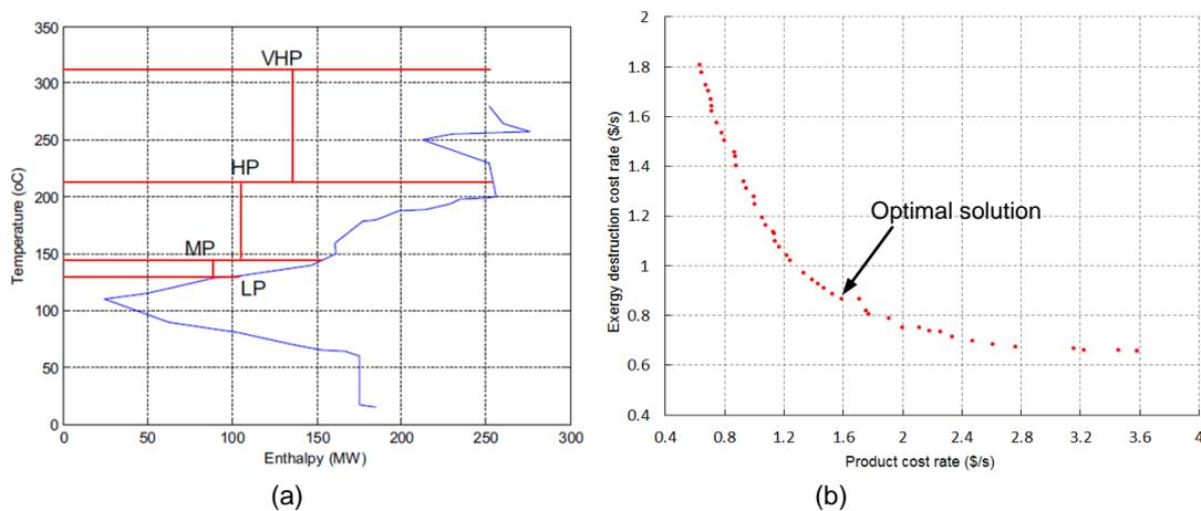
Figure 2: (a) Site utility grand composite curve (SUGCC), (b) The Pareto frontier for exergy destruction cost rate versus overall product cost rate for grassroot design
