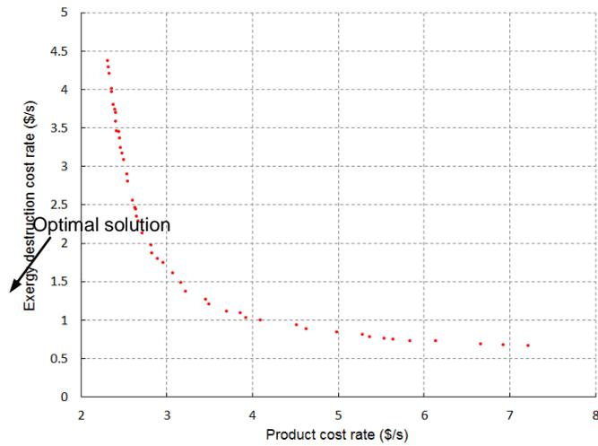
Figure 5: The Pareto frontier for exergy destruction cost rate versus overall product cost rate for retrofit design
