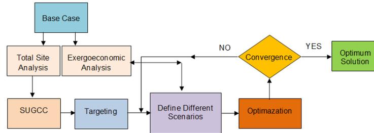
Figure 1: Algorithm of new procedure for synthesis of site utility
