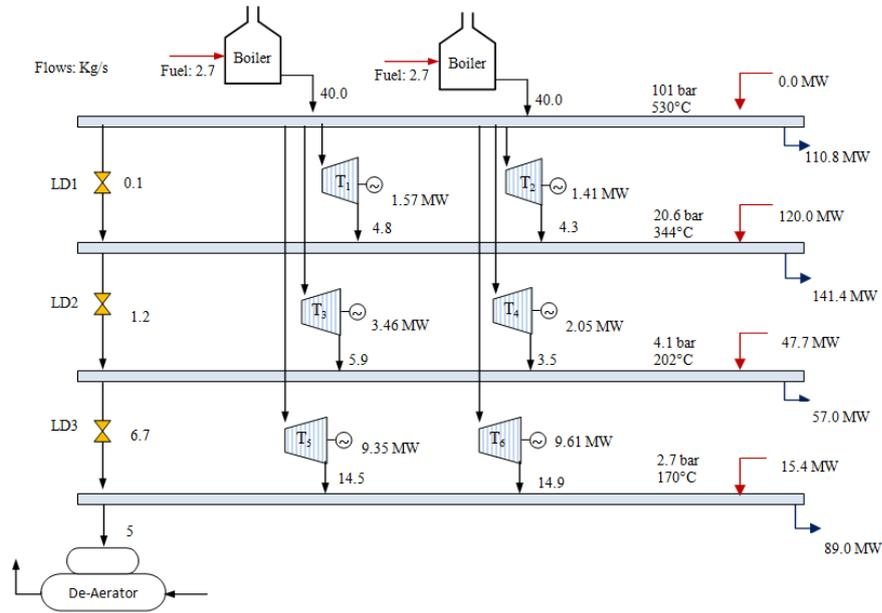
Figure 3: Optimum arrangement of steam network
