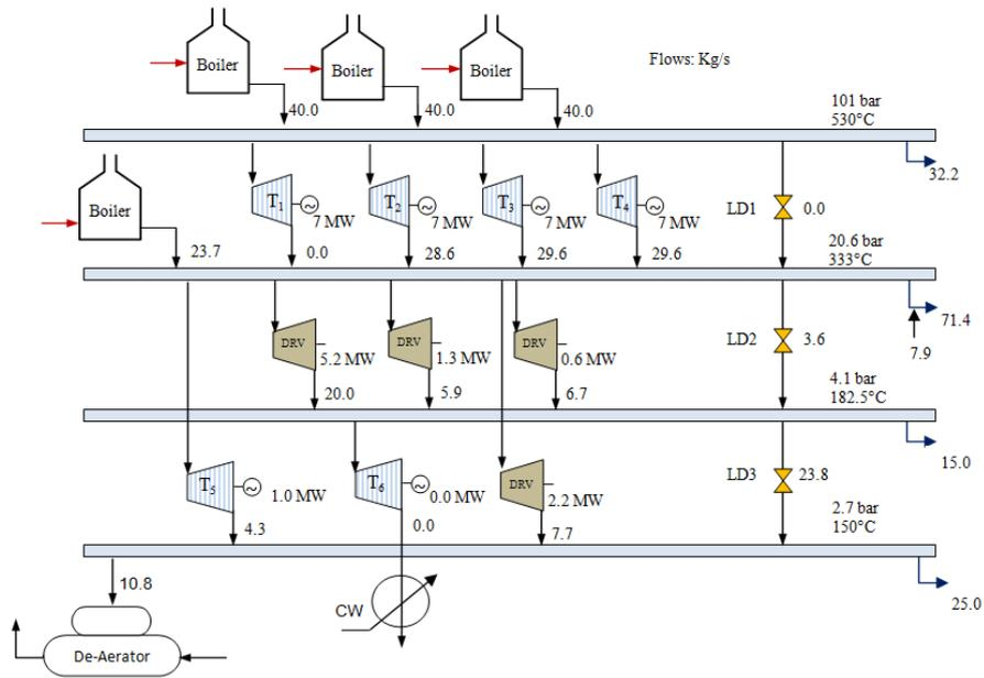
Figure 4: The operational flow sheets of the optimum case.
