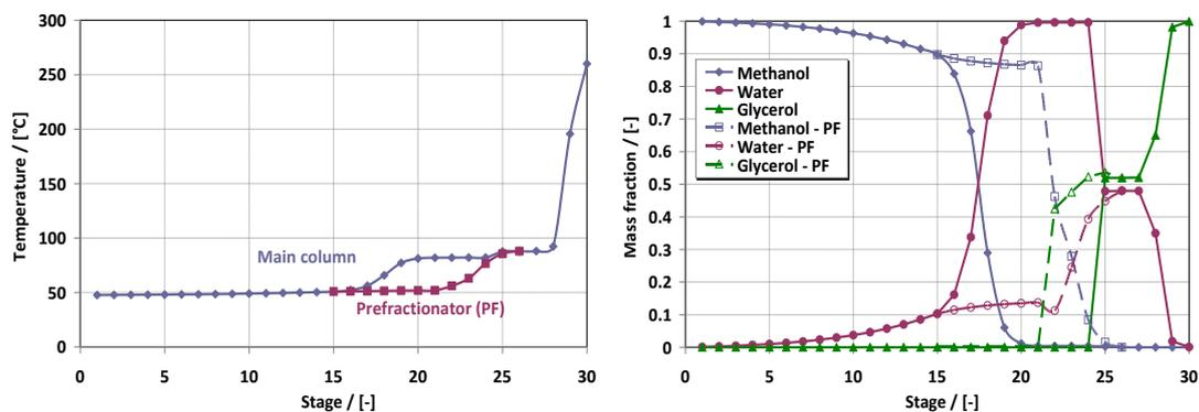
Figure 3. Temperature and composition profile in the dividing-wall column (dotted line means the pre-fractionator or the feed section of the column)
