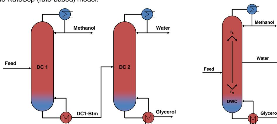
Figure 1. MeOH-water-glycerol separation in a direct sequence (left) and a dividing-wall column (right)
