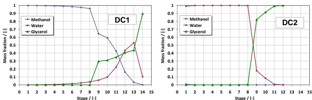
Figure 2. Composition profile in DC1 and DC2 units of the conventional direct distillation sequence
