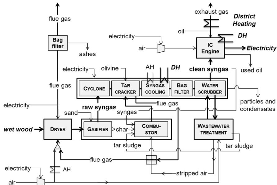
Figure 1: Overview of the modelled biomass gasification CHP plant
