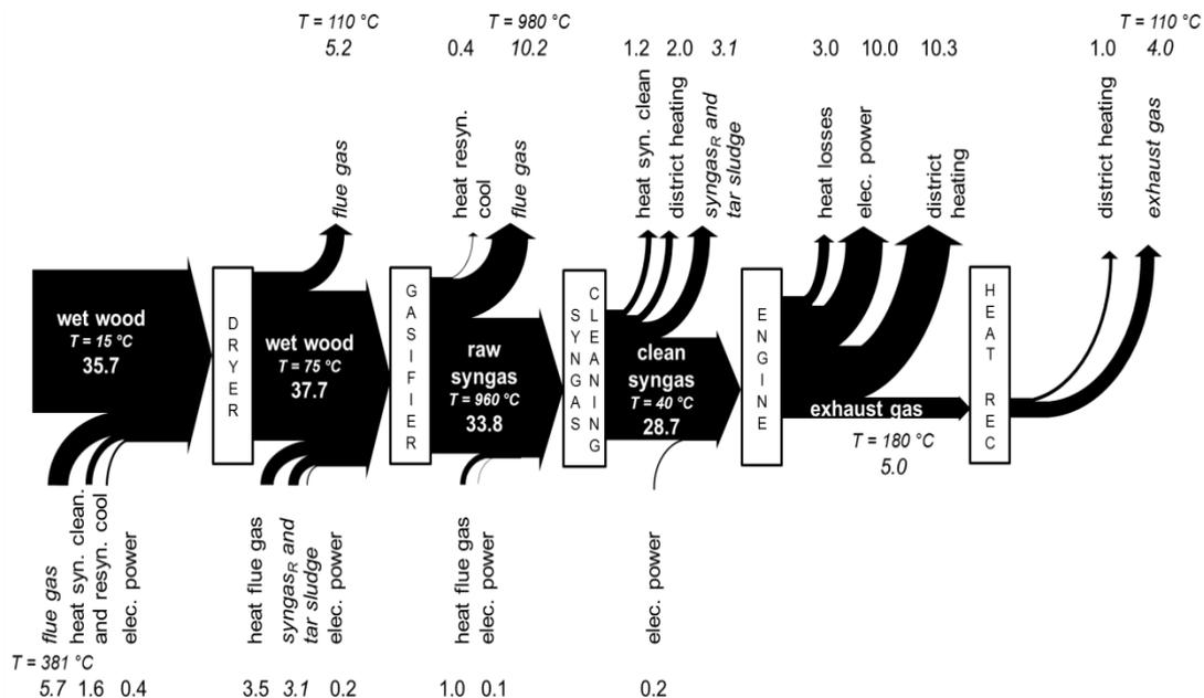
Figure 3: Sankey diagram of the energy performance of the CHP plant (heat stream unit: MW)
