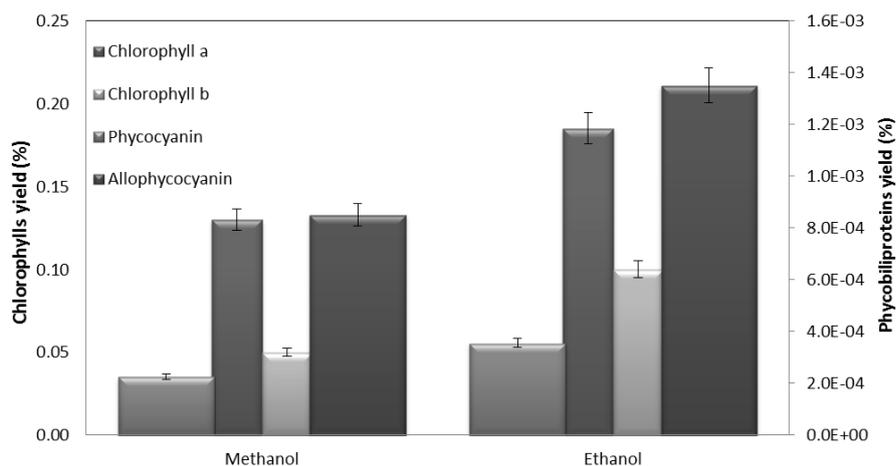
Figure 2: Effect of solvent in pigments and phycobiliproteins extraction from *Amphiprora sp.* microalgae
