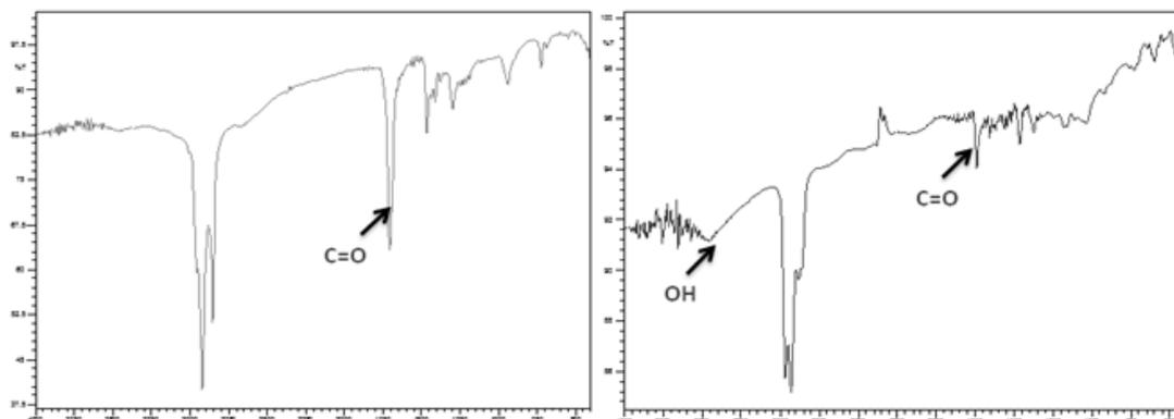
Figure 3: Comparison of FTIR spectra of hydrophobic phase from HBE and multifunctional routes
