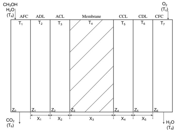
Figure 1: schematic diagram of MEA in DMFC system
