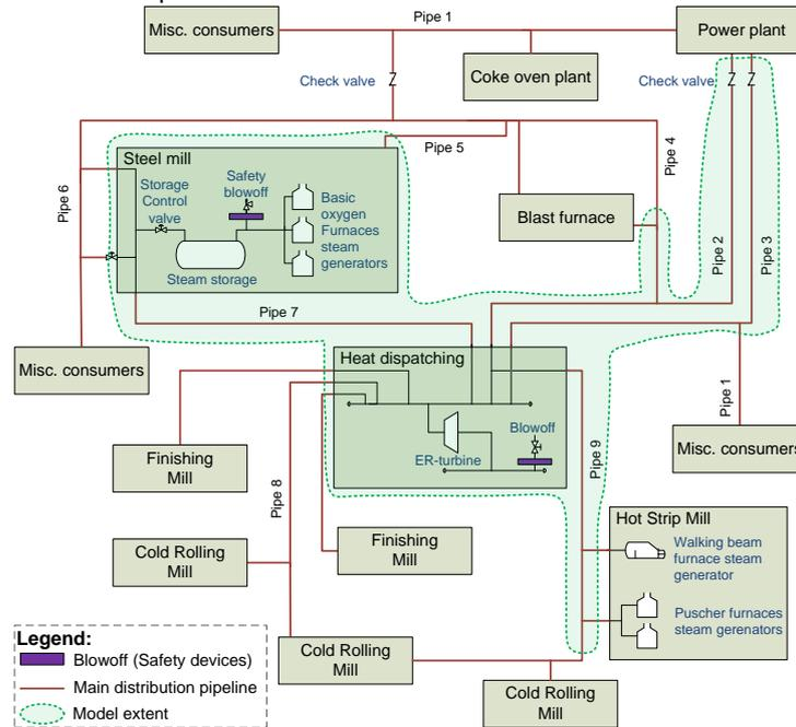
Figure 1: Schema of the steam distribution system
