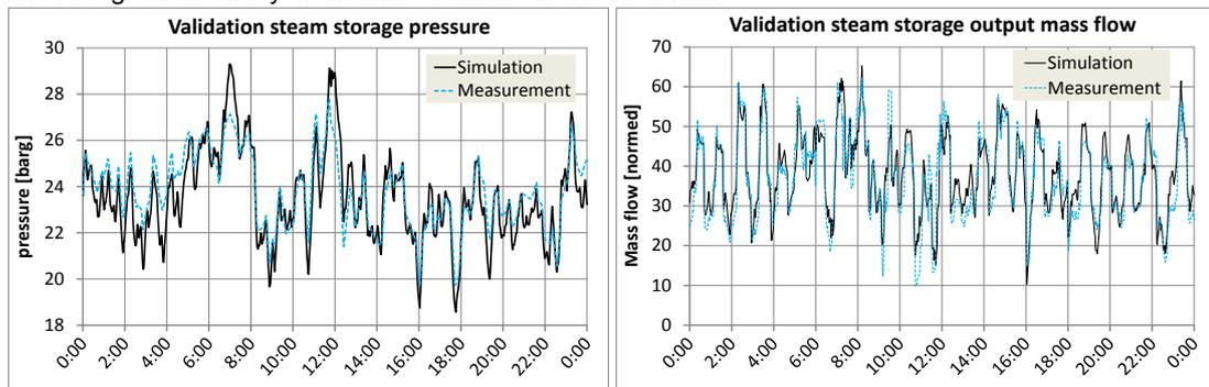
Figure 3: Validation of the steam storage system
