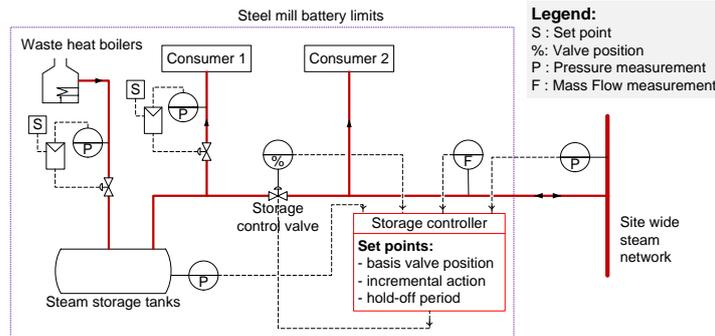
Figure 2: Modeling of the steel mill and its control loops
