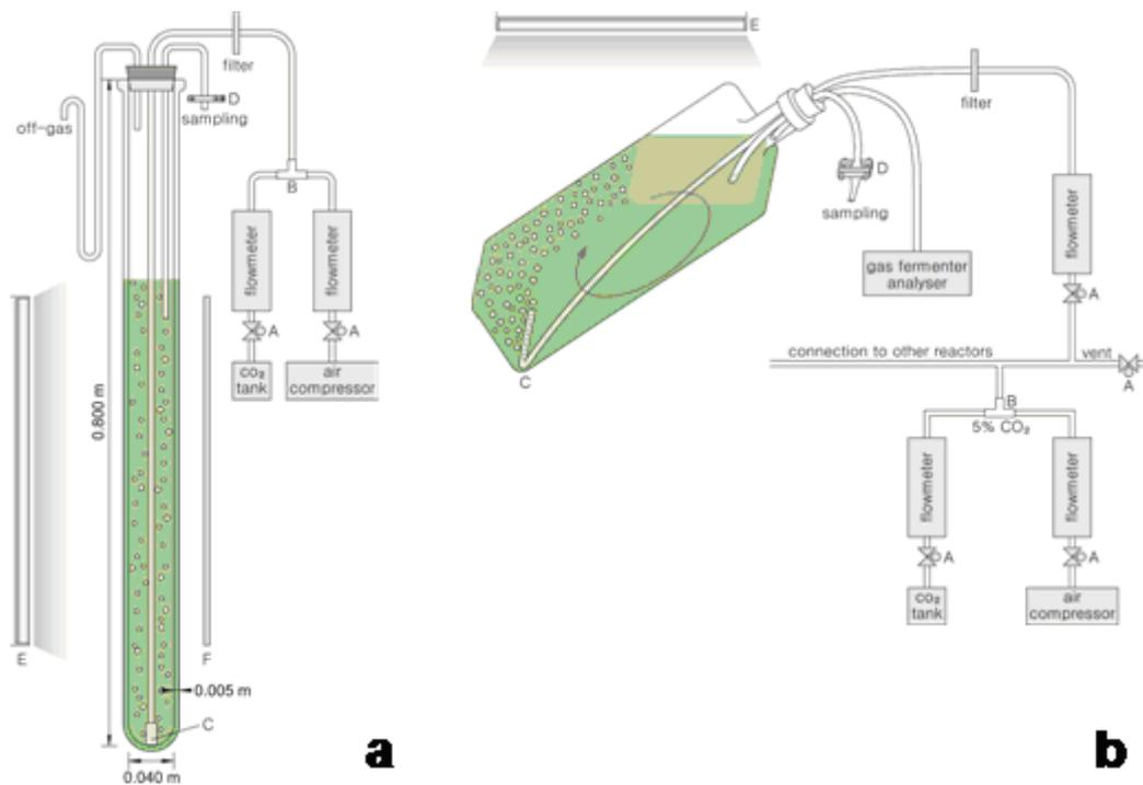
Figure 1: Sketch of the VBC (a) and of the IBC (b) photobioreactors. A) valve, C) gas diffuser, D) sterile clamp, E) light source
