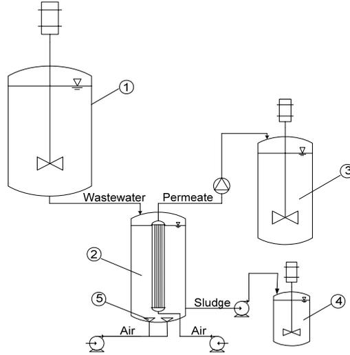
Figure 1: The experimental set-up: 1. wastewater tank; 2. membrane bioreactor; 3. permeate tank; 4. wasted sludge tank; 5. air sparger
