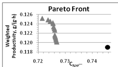
Figure 2: The Pareto front for the case without DC operation period; comparison with the point obtained with the single-objective optimization
