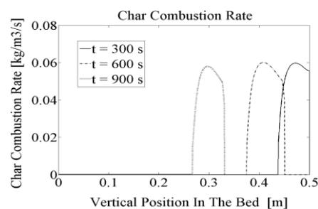
Figure 2 – Propagation of char combustion reaction front in the bed of 20-mm particles. Variable-porosity model.
