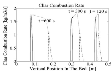
Figure 1 – Propagation of char combustion reaction front in the bed of 4-mm particles. Variable-porosity model (dash-dotted line), Constant-porosity model (solid line).
