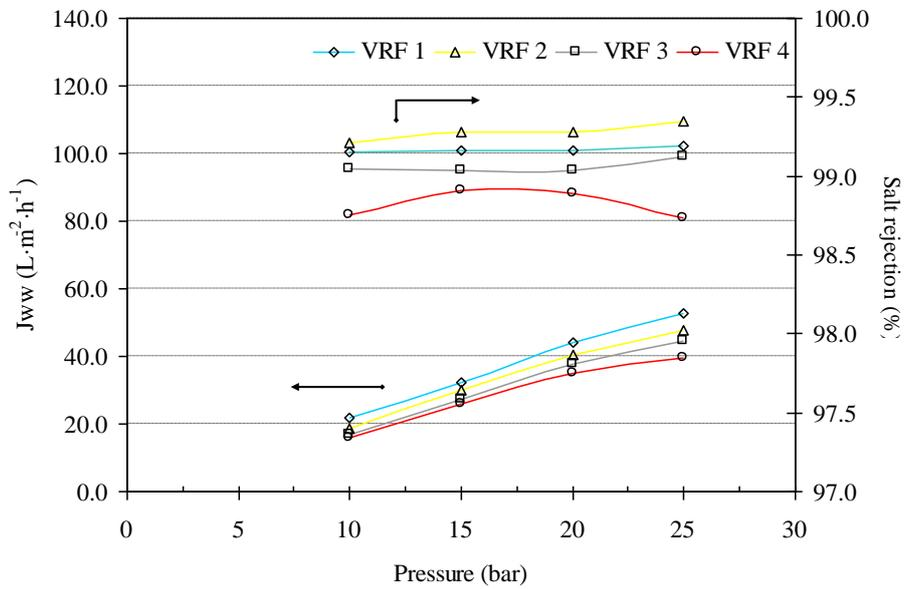
Figure 2: Relation between wastewater permeate flux rate and salt rejection with pressure (LFC1).
