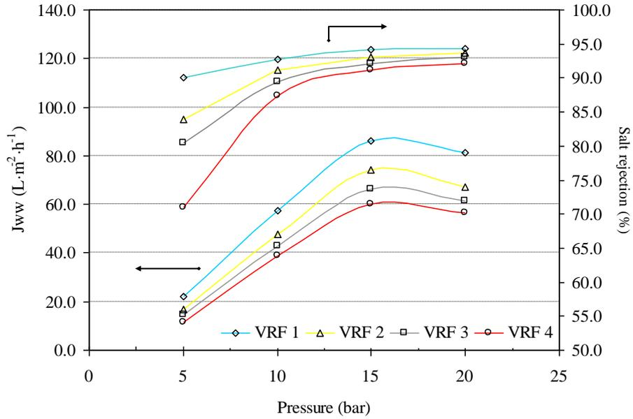
Figure 1: Relation between wastewater permeate flux rate and salt rejection with pressure (ESNA1-LF2).
