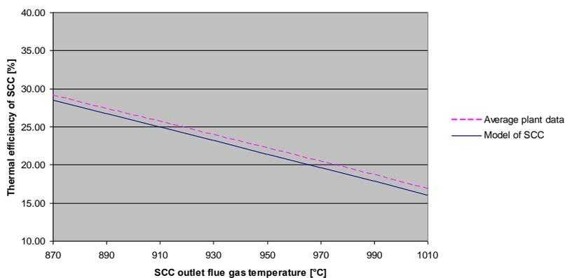
Figure 5: Thermal efficiency of SCC obtained by developed model in comparison with heat balance based on evaluation of plant data of MSWI TERMIZO Inc.
