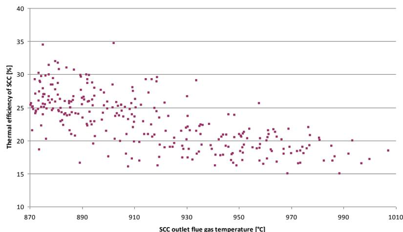
Figure 4: Thermal efficiency of SCC as function of SCC outlet flue gas temperature evaluated from plant data of MSWI TERMIZO Inc.
