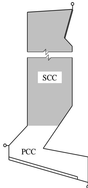
*Figure 3: Typical arrangement of SCC and PCC with travelling grate*
