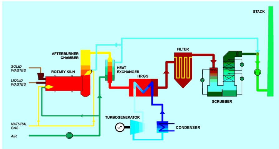
Figure 1: Typical layout of municipal or industrial waste incinerator with rotary kiln
