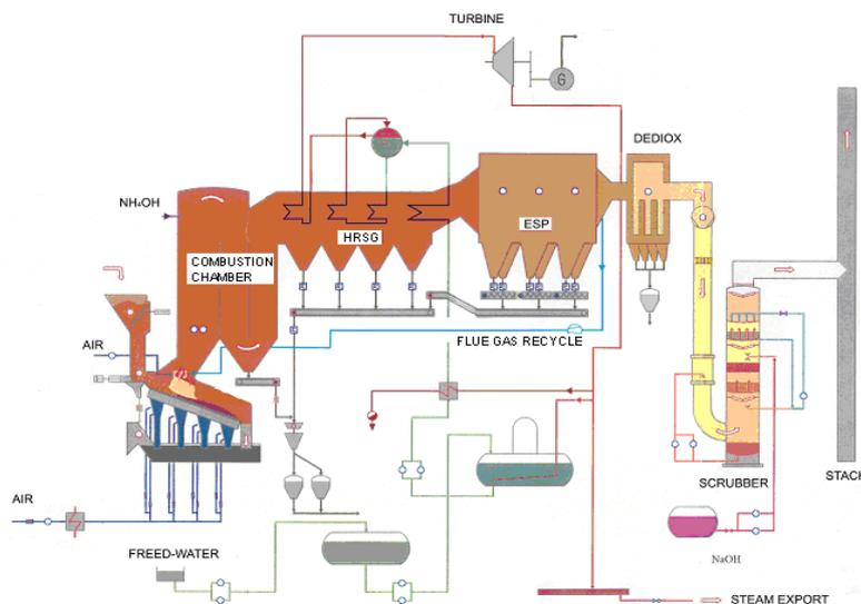
Figure 2: Typical configuration of municipal waste incinerator with fixed combustion chamber (Courtesy of TERMIZO Inc.)
