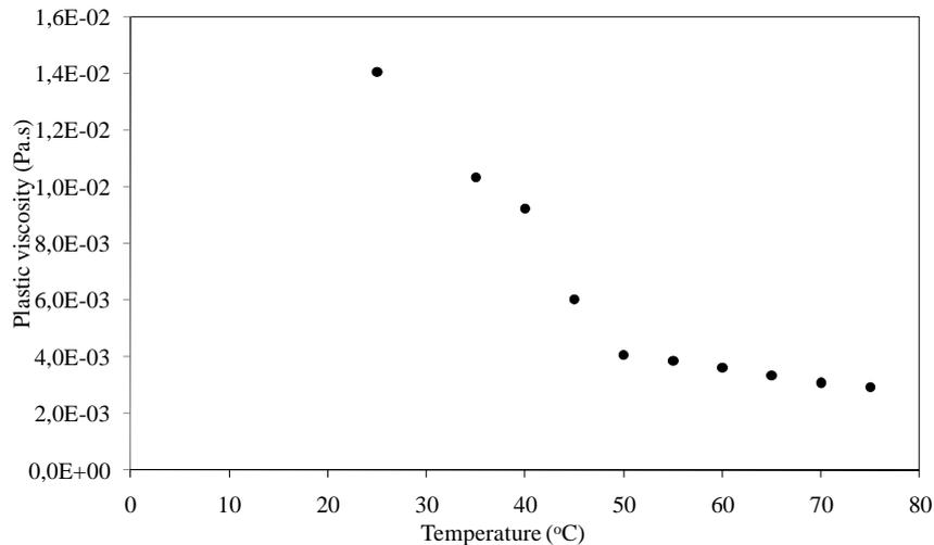
Figure 2: Plastic dynamic viscosity dependence on temperature for YS.
