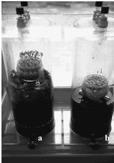
Fig. 3. No growth of L. sativum within the sludge emissions (b); good growth above a 10 cm biofilter layer (a)
