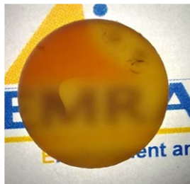
Figure 1. Translucent BaTiO 3 sintered by SPS and post-annealed in air at 800°C during 6 hours.
