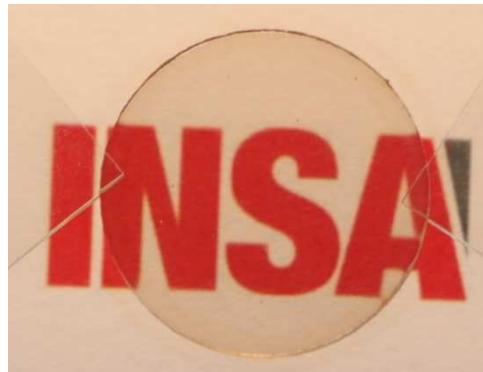
Figure 3. Spinel sample RIT = 79% at 550 nm for 1.85 mm thickness
