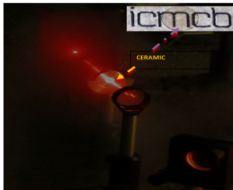
Figure 1. \text{CaF}_2 ceramic showing a good transmission in Red and infrared region tested with Laser beam wavelength 633 nm
